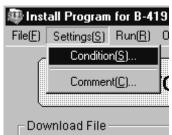
**9.** The communications setting window will appear as in figure below to allow you to change the communication parameters. Set the proper settings for Device, Parity, and Baud Rate, and click on **OK** button.
